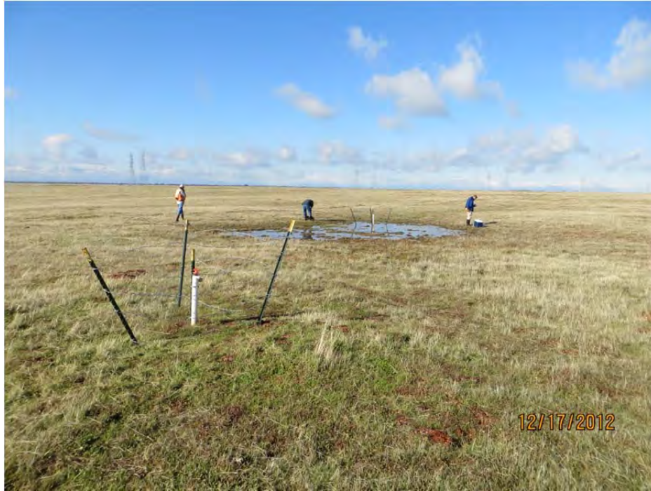
Photo IV-1. Water level standpipe installations with cattle excluders at the Agricultural Area Upland (foreground) and Depression 1 (background).
