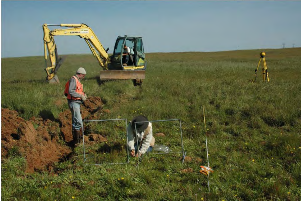
Photo IV-2. Field set-up showing the Spectre Precision Laser GL 412 level system, Track Hoe, vegetation assessment frames, and soil pit.
